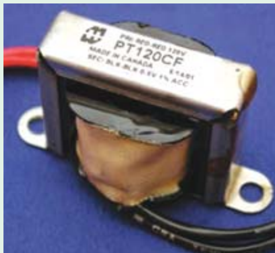
Small Potential transformer
