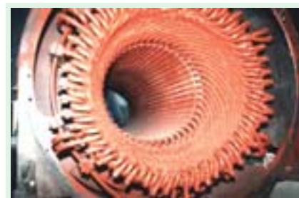
Windings of induction electric motor
