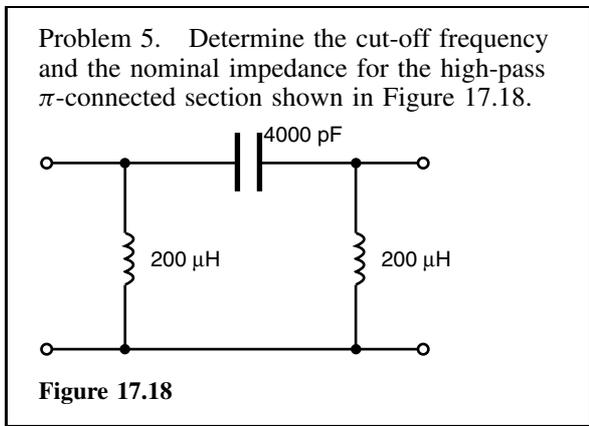
Comparing Figure 17.18 with the high-pass section of Figure 17.16(b), shows that:
