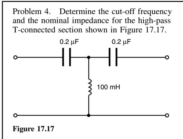
Comparing Figure 17.17 with the high-pass section of Figure 17.16(a), shows that:
